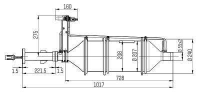
Spread of box dimensions ± 3 mm due to tolerance. Drawings with detail and connection dimensions as PDF and DXF can be found at www.HATZ-DIESEL.com.
